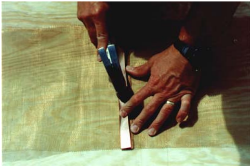
Illustration 2.51 Splice Plate and fold flattened using hammer.
