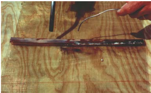
Illustration 2.52 Soldering of Splice Plate and Z Mesh.
